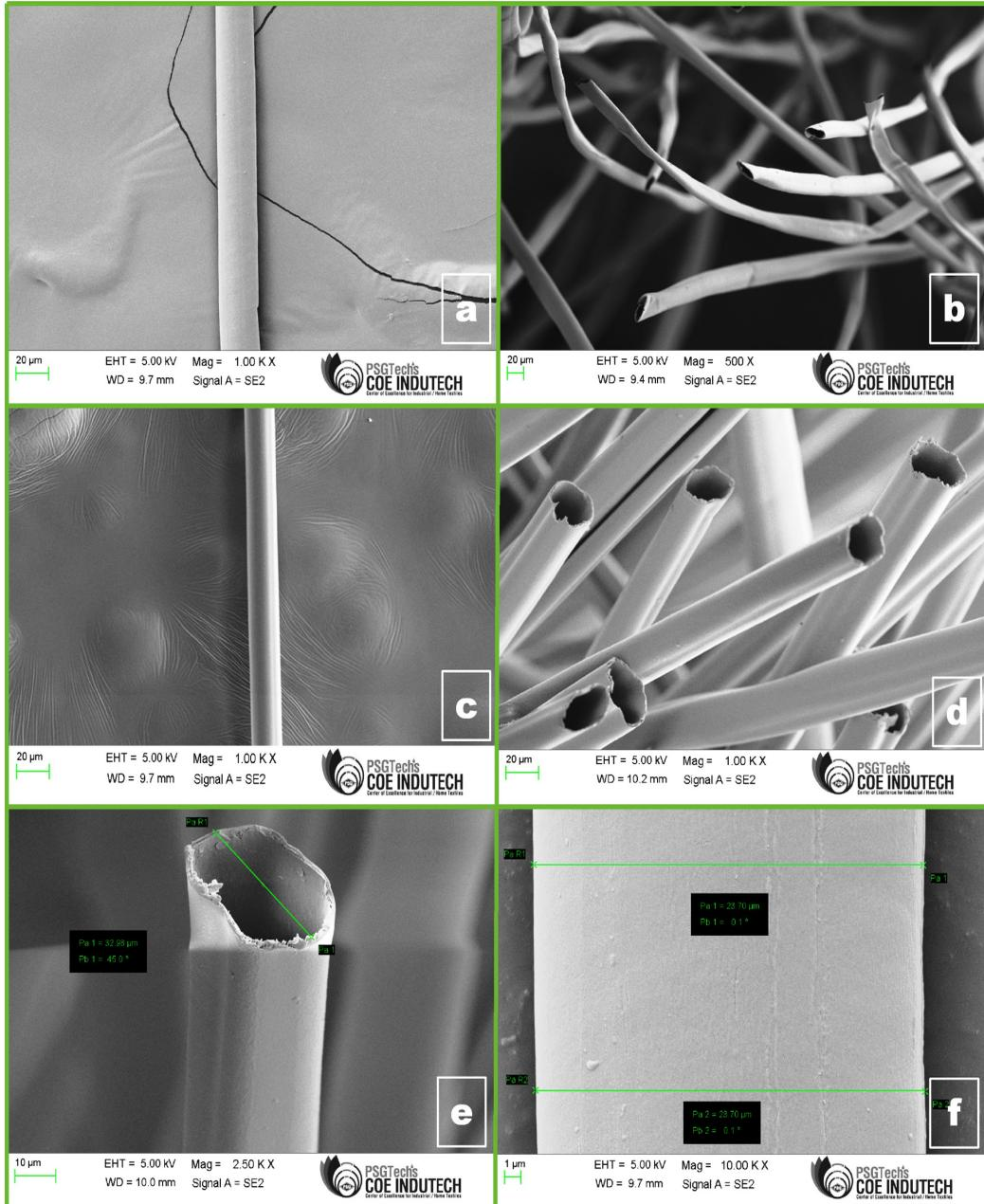
Figure 5. SEM images of (a, c) Longitudinal morphology of *Wrightia tinctoria* (WT) and *Cebia pentandra* (CP), (b, d) Cross-sectional morphology of WT and CP, and (e, f) Diameter of WT and CP
