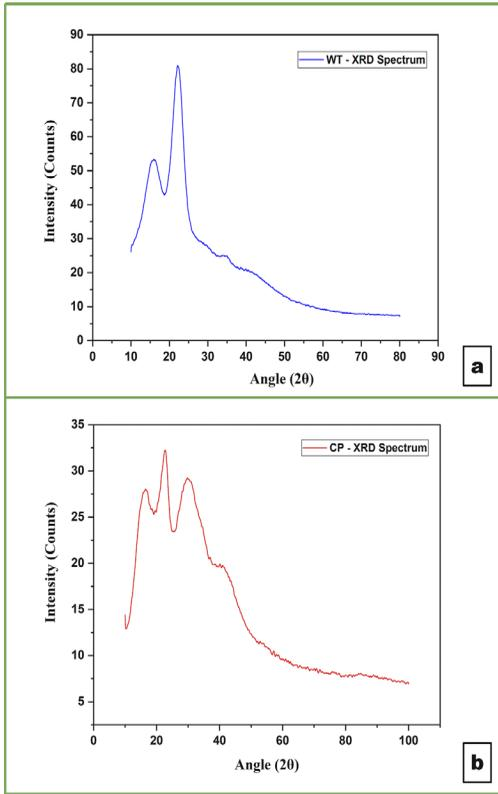
Figure 3. X-ray diffraction spectroscopy of (a) *Wrightia tinctoria* (WT) and (b) *Cebia pentandra* CP fibers
